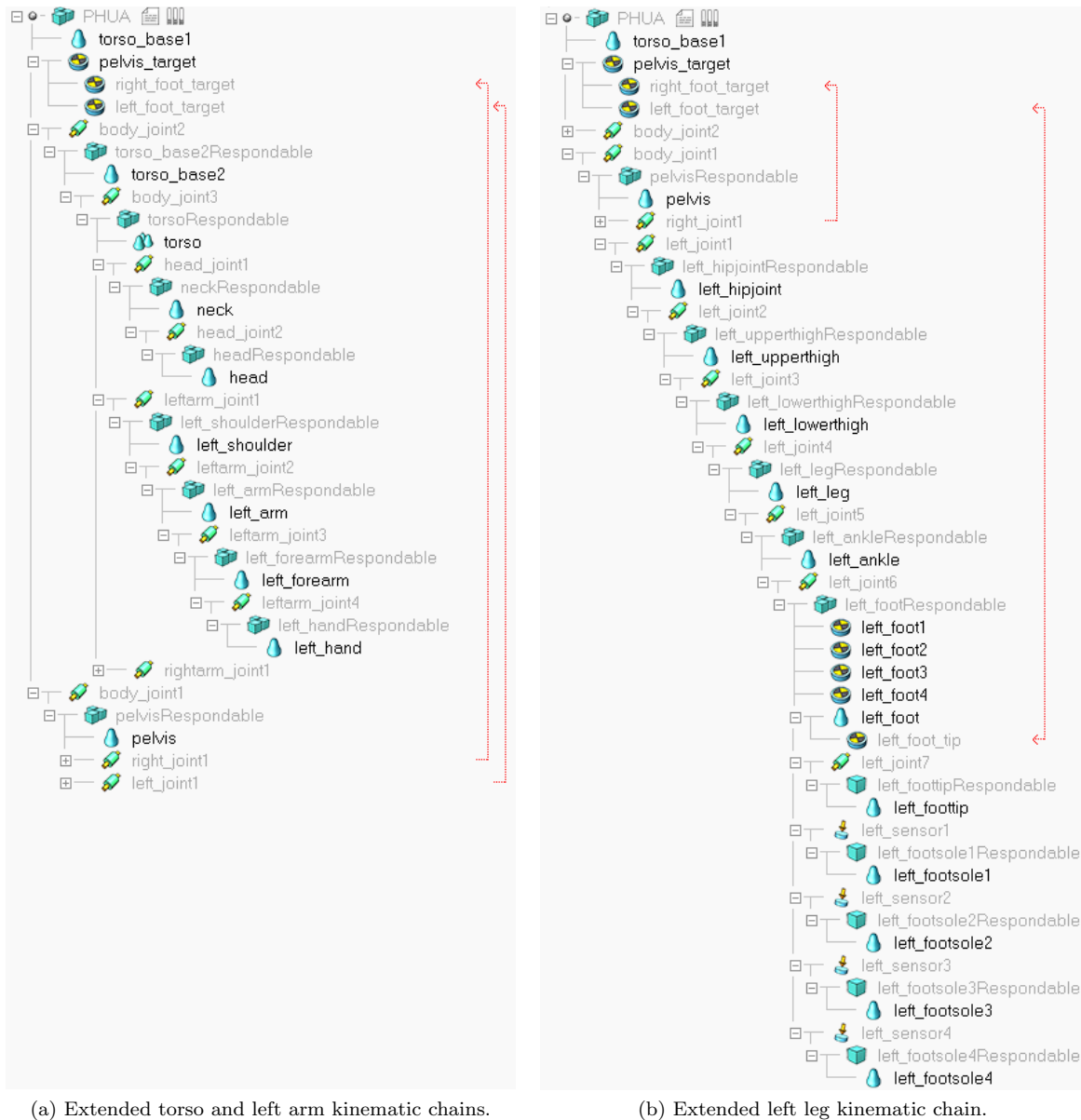
Figure 2.12: V-REP model kinematic chains construction, detailing the "tip-target" inverse kinematics links.
