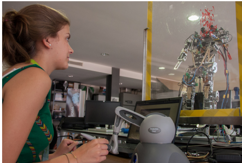
Figure 4.4: Teleoperation of the robot arm with force feedback [1].
